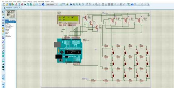
**Fig.3 Representation of no fault condition using simulation**
