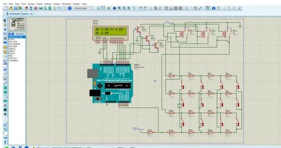
**Fig.4 Representation of faulty condition in all three phases using simulation**
